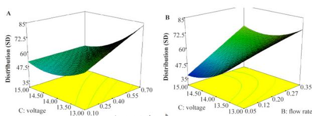
Figure 2. Effects of voltage and concentration: A) as well as voltage and flow rate; B) on nanoparticles size distribution.
