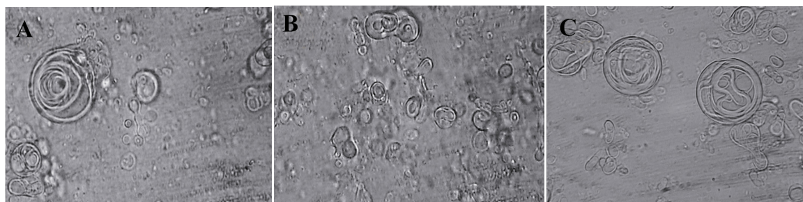
Figure 2. Morphological micrographs of niosomes ( \times 400 ): A) formulation composed of Span 20/Tween 20/Cholesterol; molar ratio (m.r) 35:35:30, B) formulation composed of Span 60/Tween 60/Cholesterol; m.r 35:35:30 and C) formulation composed of Span 80/Tween 80/Cholesterol; m.r 35:35:30.
