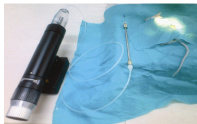
Figure 1. Manual piston pump (Cell Tram Oil®) used in mouse embryo transfer
